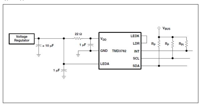
$V_{BUS}$  in the above figure refers to the  $I^2C$  bus voltage which is either  $V_{DD}$  or 1.8 V. Be sure to apply the specified  $I^2C$  bus voltage shown in the Available Options table for the specific device being used.
