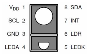
Figure TMD3782 – 4: Pin Description
